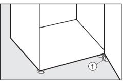
■ **Ensure** that you unscrew adjusting foot ① from the hinge plate until it sits on the floor. Then unscrew the foot by a further 90°.
